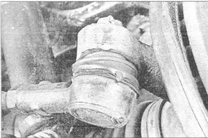
17.6b The grease oozing from this tie-rod end boot indicates that it needs replacing
