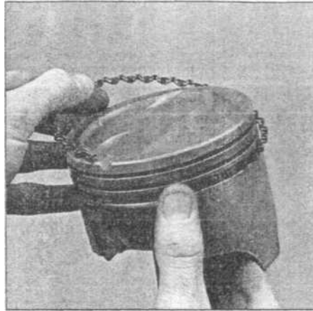
21.9a Install the three-piece oil control ring first, one part at a time, beginning with the spacer/expander ...
