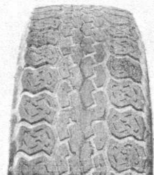
FEATHERING DUE TO MISALIGNMENT
