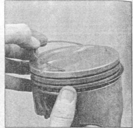
21.9b ... followed by the side rails - DO NOT use a piston ring installation tool to install the oil ring rails
