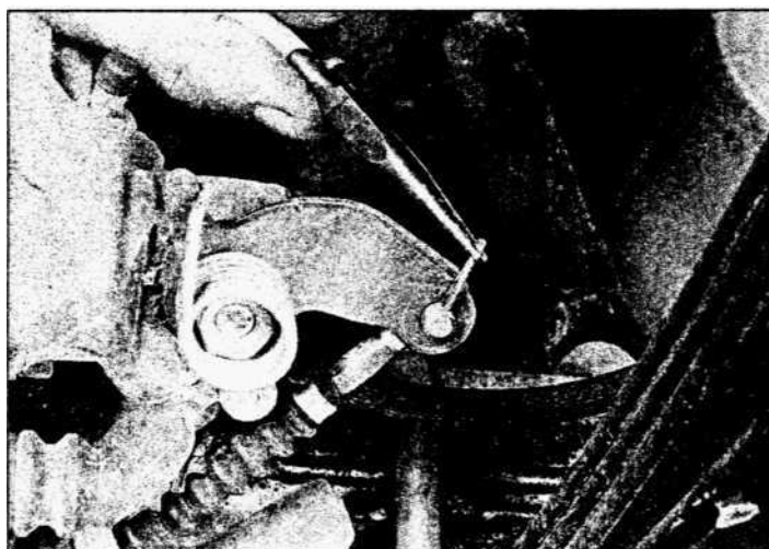
2.11 Use pliers to pull the cotter pin out of the retaining pin, then disconnect the parking brake cable
