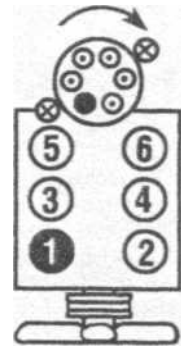
Cylinder locations and distributor rotation
