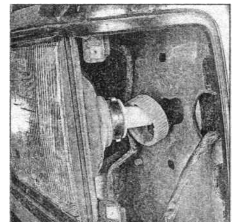
10.9 Unscrew the retaining collar and slide it back so the bulb can be pulled out of the housing
