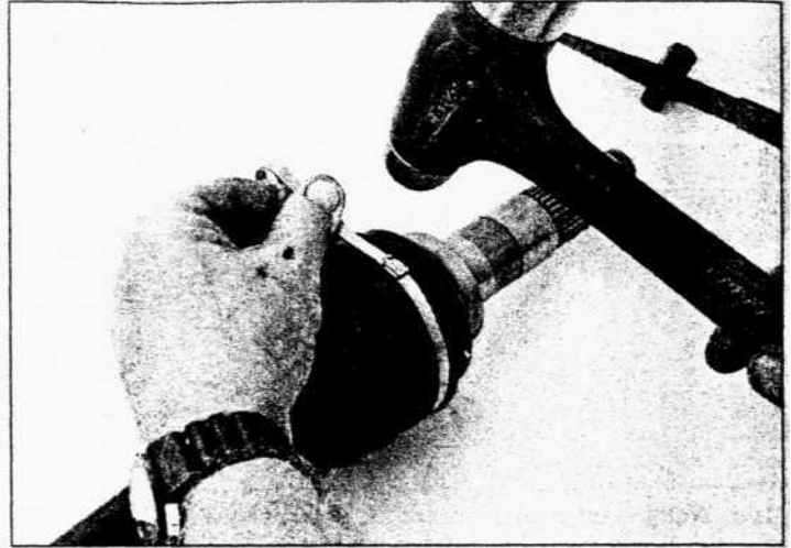
20.16b . . . peen over the locking tabs . . .
