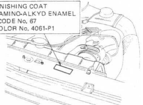
The paint code ID plate is usually located on the radiator support
