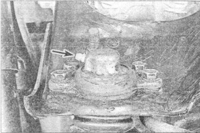
16.3a Upper balljoint grease fitting (arrow)
